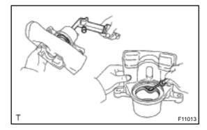
(b) Use compressed air to remove the piston from the cylinder.
